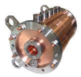
Another kind of diagnostic components for the characterization of the beam are the **RF-deflectors**. This devices are used at SPARC for the determination of the bunch length.
