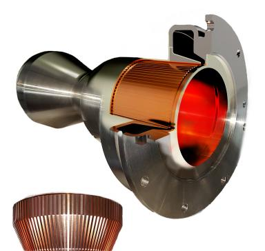
96 channels up to 0.87 mm wide run along the walls of the combustion chamber and allow for liquid methane heating, at 150 bar of pressure. The results of the pressure test are really encouraging, and a new prototype will be fire-tested soon in 2019.
